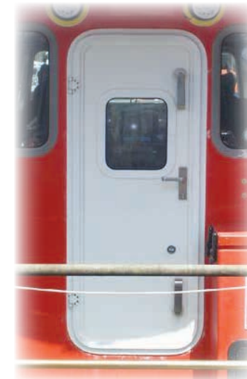
Independently operated dog handles
