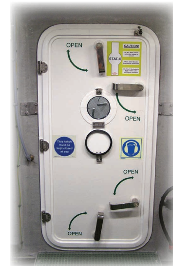
Independently operated dog handles
