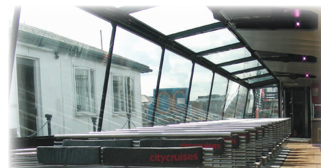
Internal view of minimal framework, a major design feature of this vessel
